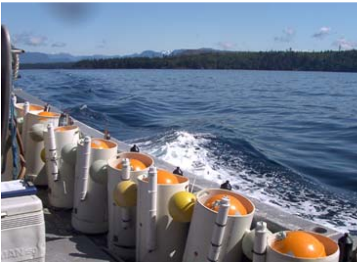
Deployment of pop-up moorings with receivers & acoustic releases
