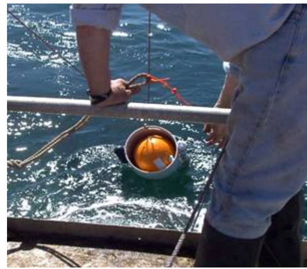
Deployment of pop-up moorings with receivers & acoustic releases
