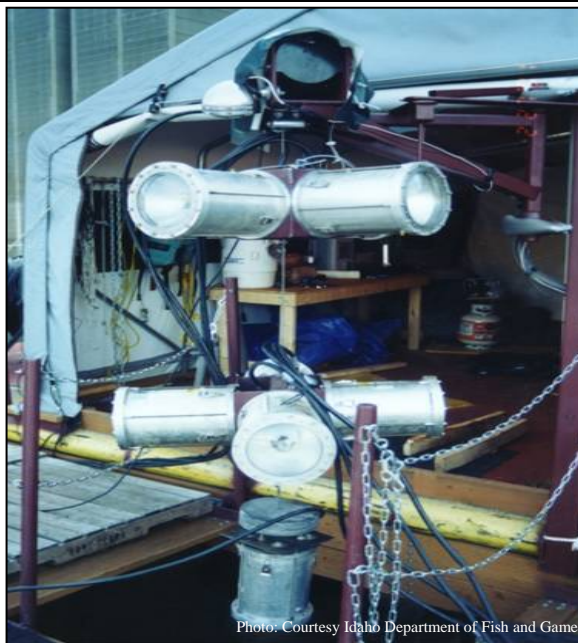
Strobe light array used to direct fish away from Dworshak Dam.
