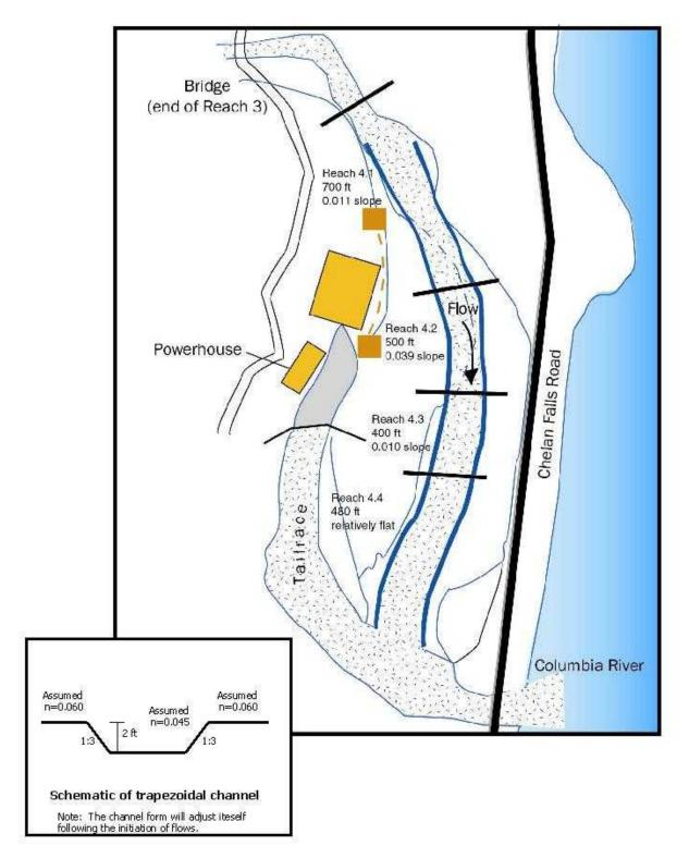
Figure 3. Schematic diagram of the subreaches of Reach 4, including an example of the trapezoidal channel
