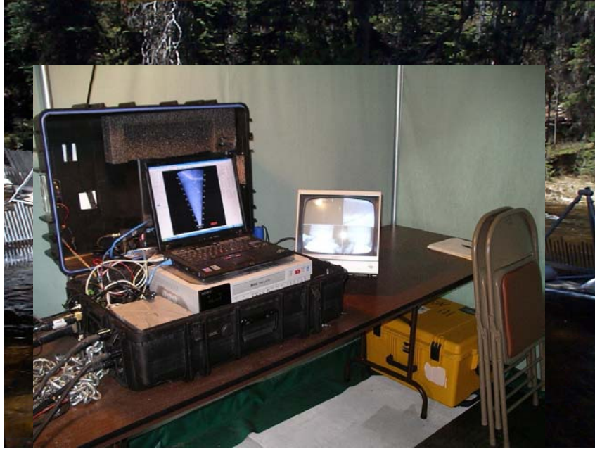
Figure 4. Topside box with laptop computer that collects DIDSON files on an external hard drive, and quadplexes optical camera data with the DIDSON signal on a VHS tape for validation studies.
